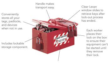
The supervisor locks out the energy sources and drops the keys into the box.
